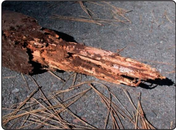
*Figure 173. Damage to sign post caused by termites in Oak Creek Canyon, Arizona.*
